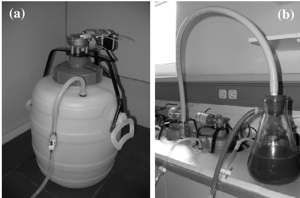
Figure 3.2 Experimental set up of anaerobic digestion tests showing a a 20-l polyethylene batch digester with direct current motor on top for the stirring unit and b a continuously working stirrer tank digester in a water basin with the additional apparatus for removal of digester fluid.
