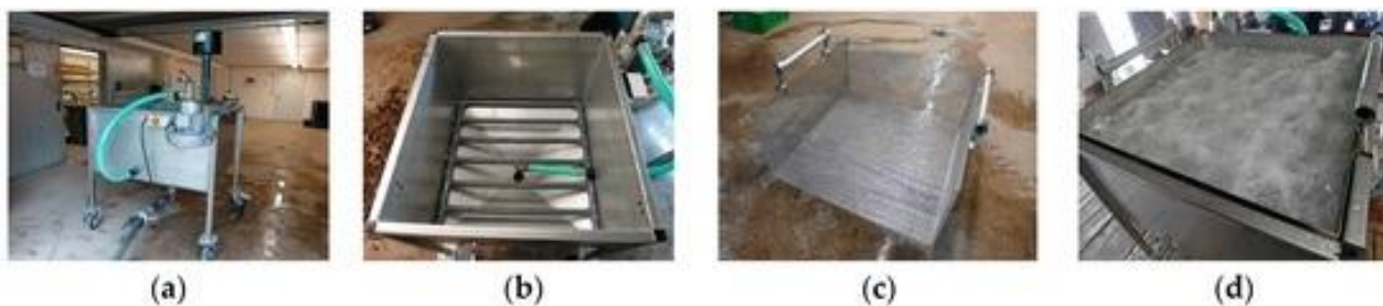
Figure 3.2 Foliage cleaning machine from the side (a); pipes and water outlet valve in the bottom (b); sieve basket (c) and in operation (d).
